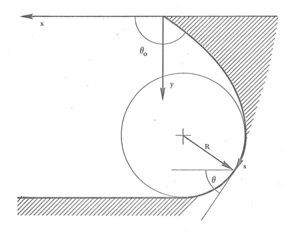
Figure 3. Geometry of the cutting surface. The jet enters with a positive rake (cf. Section 8).
